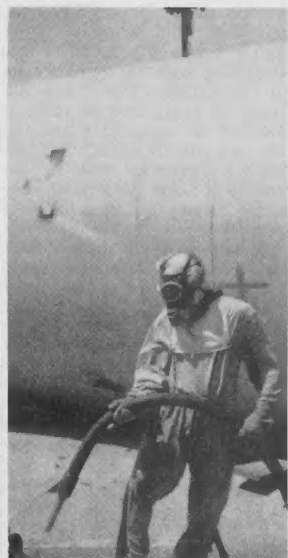
SANDBLASTER WEARING protective gear at work. SANDBLASTER NA trabao.
